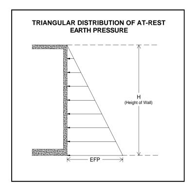
In addition to the recommended earth pressure, the upper ten feet of the retaining wall adjacent to streets, driveways or parking areas should be designed to resist a uniform lateral pressure of 100 pounds per square foot, acting as a result of an assumed 300 pounds per square foot surcharge behind the walls due to normal street traffic. If the traffic is kept back at least ten feet from the retaining walls, the traffic surcharge may be neglected.
