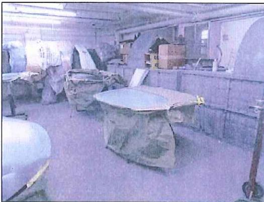
Photo #14: Automotive body parts prepped for painting in paint booth.
