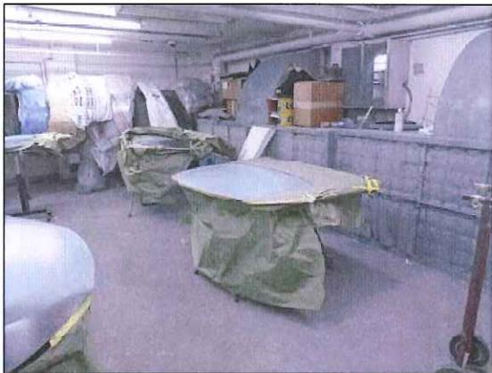
Photo #14: Automotive body parts prepped for painting in paint booth.
