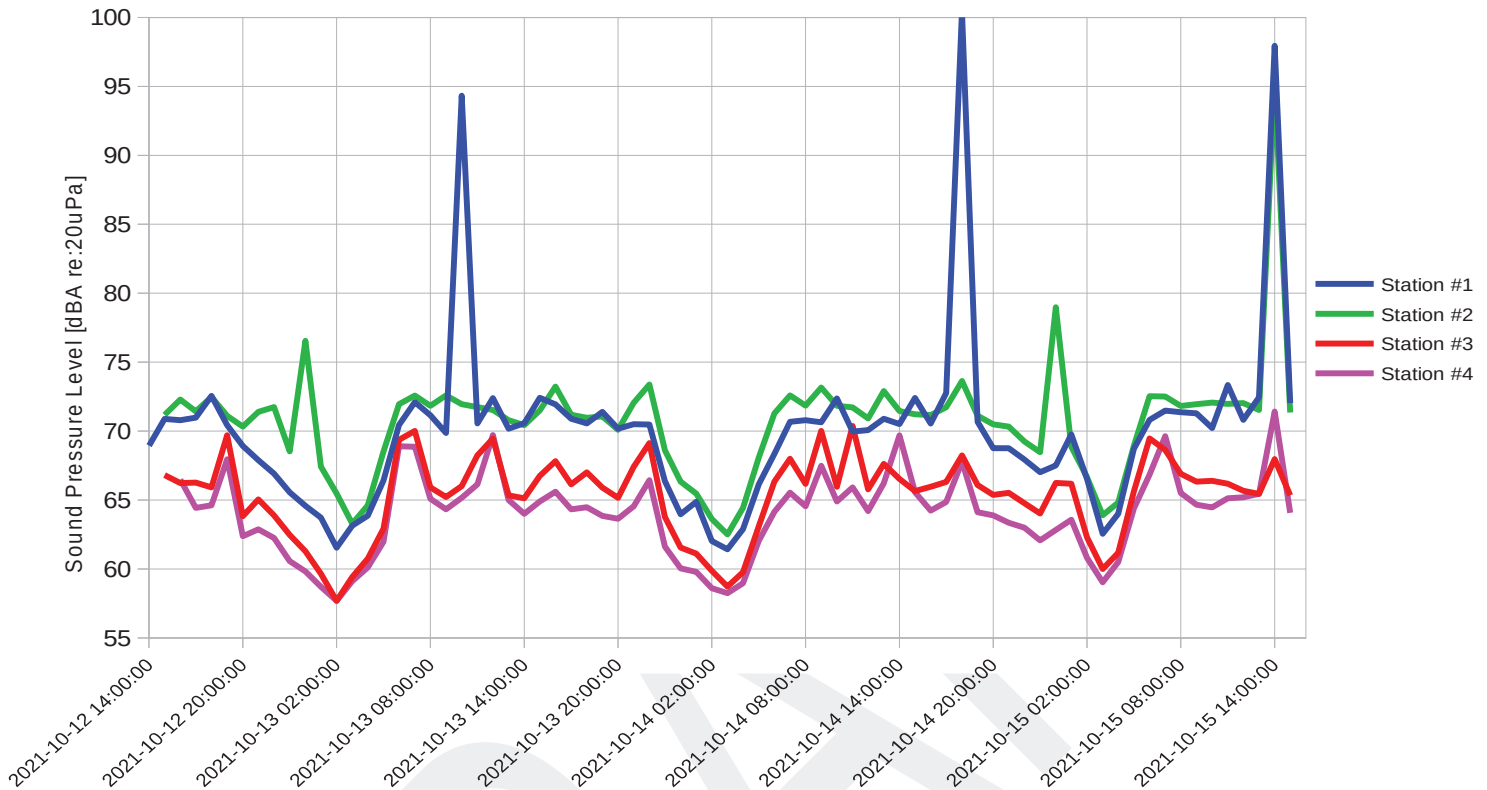
Figure 9: Hourly equivalent A-weighted (LAeq,1hr) ambient levels measured at 72-hour monitoring stations. High hourly equivalent levels at Station #1 are believed to be caused by loud braking of either Metro busses or garbage trucks, both of which were observed frequently on Riverside Drive.
