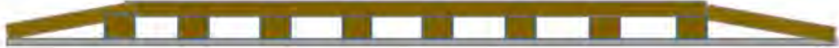
Diagram: Side view depiction of elevated road segment (rectangle with vertical lines) with barrier fencing (lines) and openings for toad passage underneath (solid rectangles); not to scale.
