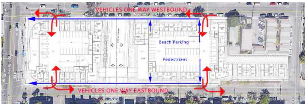
FIGURE 19 – UNSAFE PROJECT VEHICLE/VEHICLE AND PEDESTRIAN/VEHICLE MOVEMENT CONFLICTS
