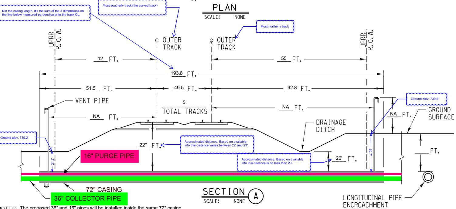
NOTES: The proposed 36" and 16" pipes will be installed inside the same 72" casing.
