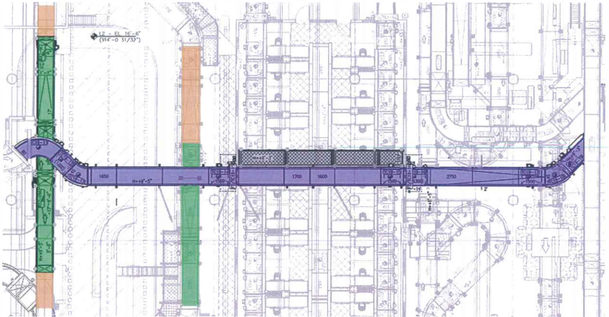
TC 19 Concept Layout. Purple is TC-19 conveyor, green is base scope conveyor requiring replacement, orange is base scope conveyor requiring modification, grey is catwalk.
