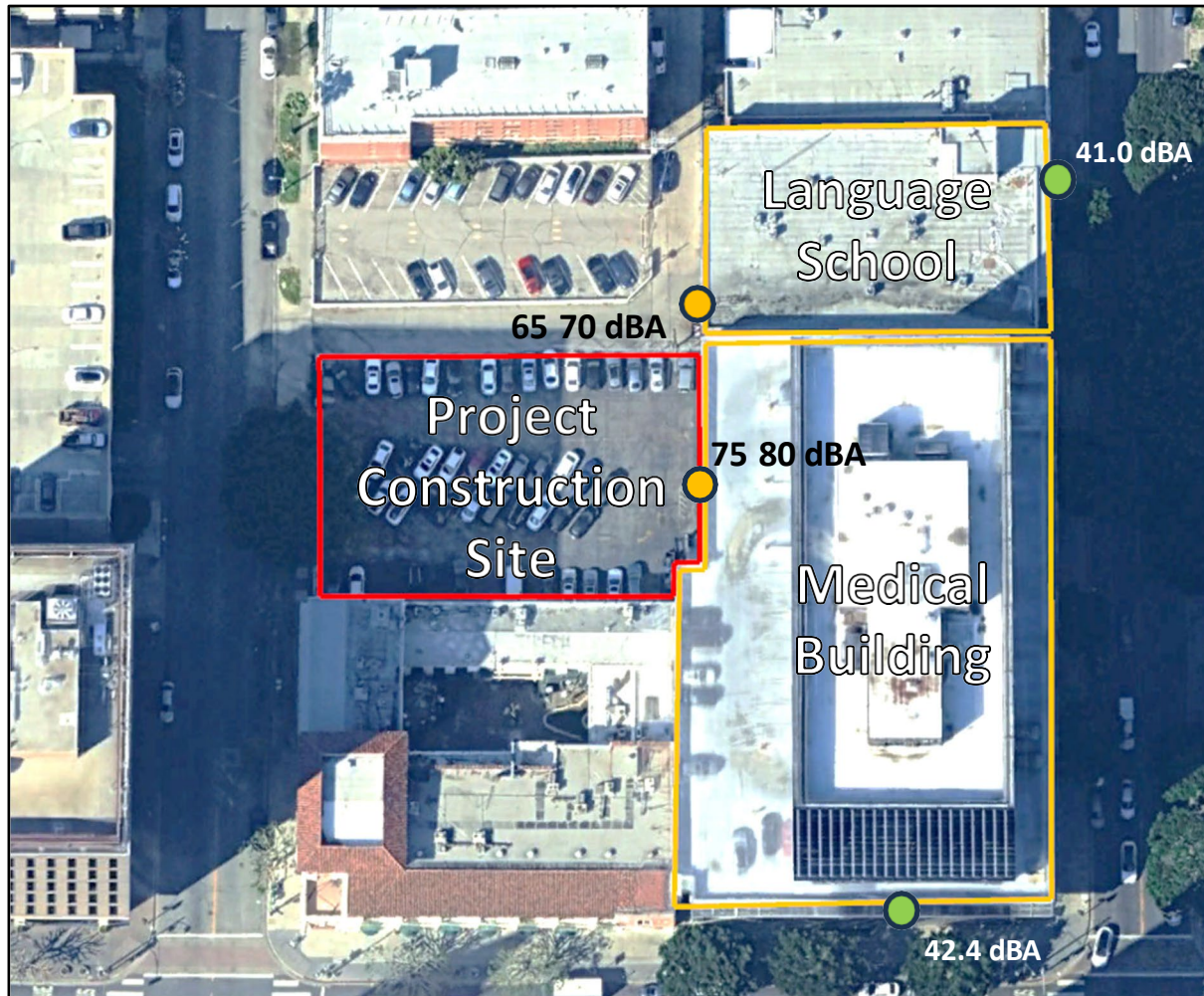
Figure 2. Construction Noise Levels at Adjacent Noise Sensitive Receptors
