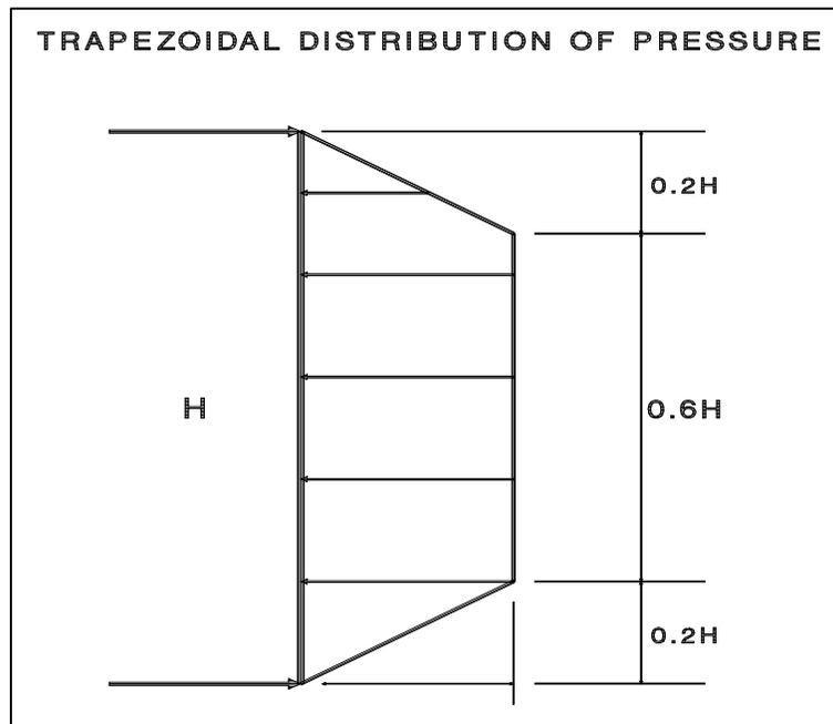
Where a combination of sloped embankment and shoring is utilized, the pressure will be greater and must be determined for each combination. Additional active pressure should be applied where the shoring will be surcharged by adjacent traffic or structures. Where a combination of sloped embankment and shoring is utilized, the pressure will be greater and must be determined for each combination.
