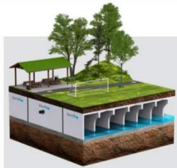
Figure 2: typical Infiltration Gallery (Source: StormTrap)
