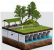
Figure 2: Typical Infiltration Gallery (Source: StormTrap)
