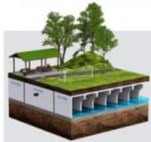
Figure 2: Typical Infiltration Gallery (Source: StormTrap)
