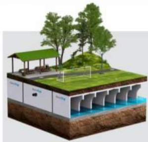
Figure 2: typical Infiltration Gallery (Source: StormTrap)
