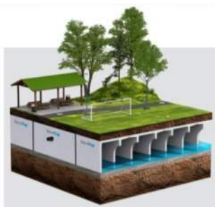
Figure 2: typical Infiltration Gallery (Source: StormTrap)
