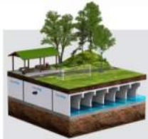
Figure 2: Typical Infiltration Gallery (Source: StormTrap)
