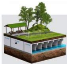
Figure 2: Typical Infiltration Gallery (Source: StormTrap)
