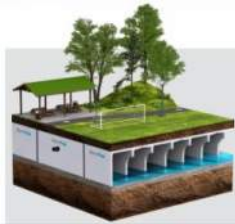
Figure 2: Typical Infiltration Gallery (Source: StormTrap)
