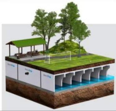
Figure 2: typical Infiltration Gallery (Source: StormTrap)
