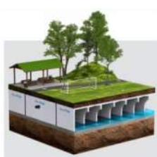
Figure 2: Typical Infiltration Gallery (Source: StormTrap)
