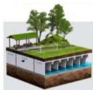
Figure 2: Typical Infiltration Gallery (Source: StormTrap)
