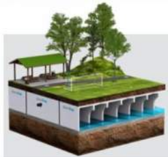
Figure 2: Typical Infiltration Gallery (Source: StormTrap)
