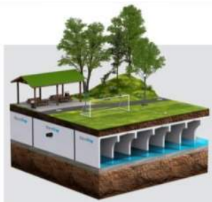
Figure 2: typical Infiltration Gallery (Source: StormTrap)
