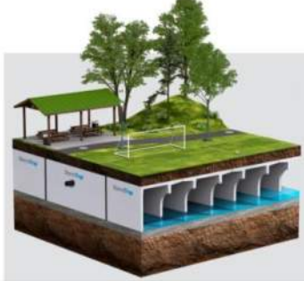
Figure 2: Typical Infiltration Gallery (Source: StormTrap)
