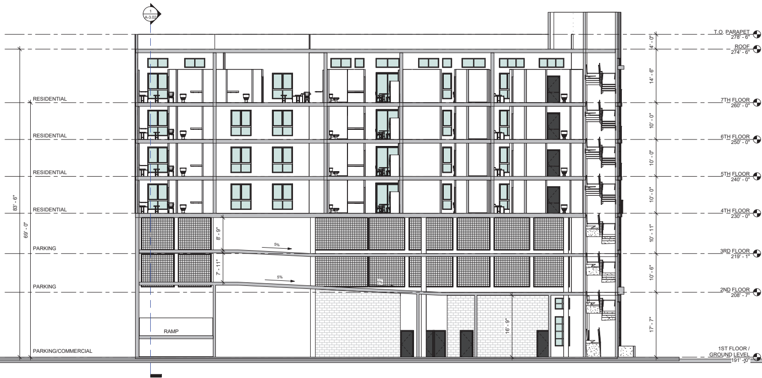
BUILDING SECTION - AA | SCALE: 1/8" = 1'-0" ①
