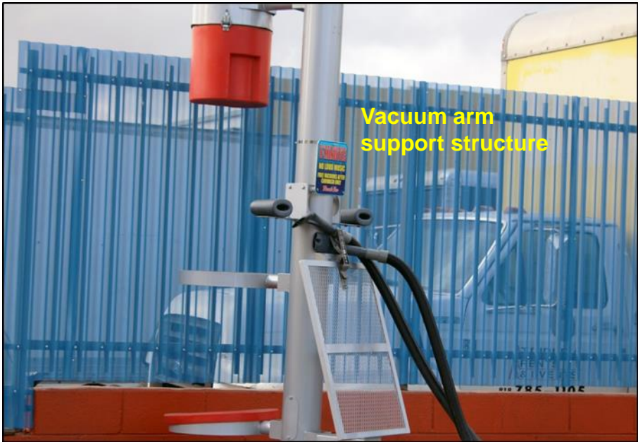
This picture shows how the nozzles were secured to the vacuum arm support when testing the noise impact from all nozzles simultaneously. The nozzles were all mounted facing the Halbrent Ave. microphone which represents a worst case situation (ref. Graphic 2.9 ).
