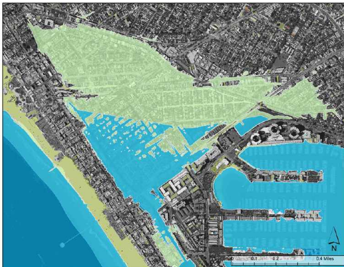
Figure 3.5: Comparison of CoSMoS 3.0 and Adapt LA - Potential Inland Flooding Areas
