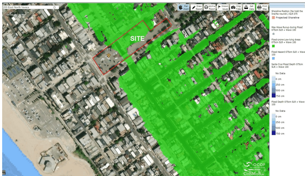
Figure 4. CoSMoS output for 2.5 feet of SLR at the site in the Venice Area.
