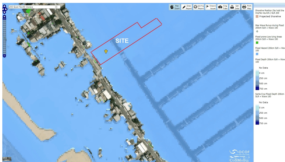
Figure 6. CoSMoS output for 6.6 feet of SLR at the site in the Venice Area.
