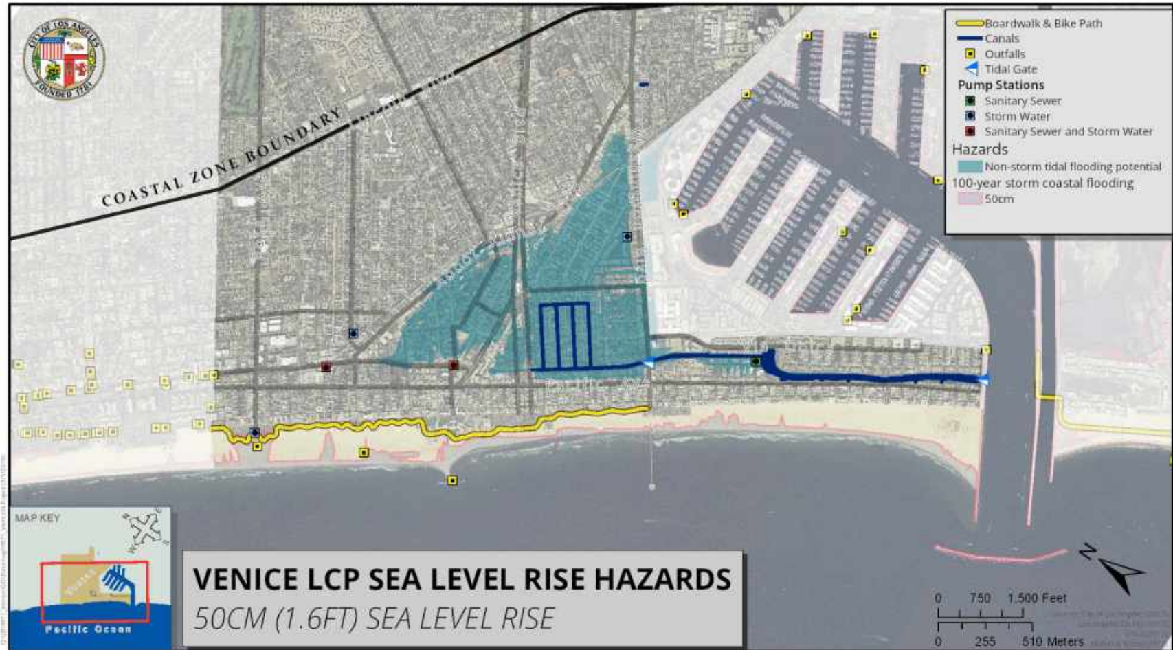
Figure 5.2: Coastal and Inland Flooding for 1.6-ft Sea Level Rise Scenario
